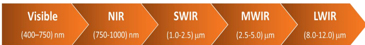
Figure 1: The typical definition of the various sub-regions of the electromagnetic spectrum, covering visible through to infrared wavelengths.
