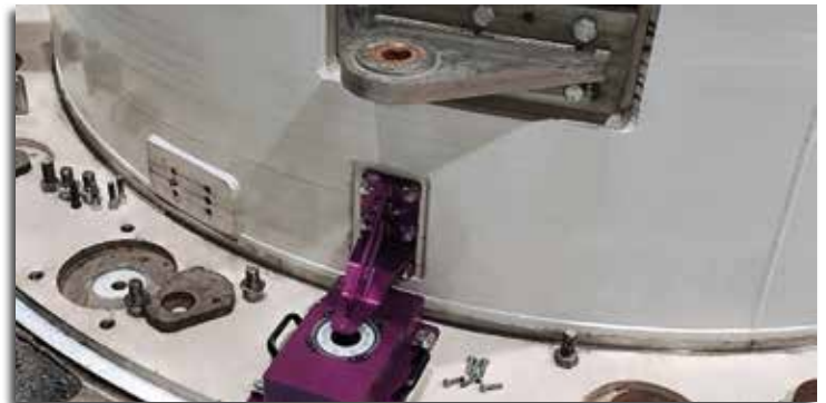
Camera and light placed on the pallet and target on the booster
