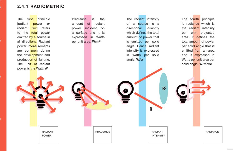
The photometric equivalent of radiant power is luminous power, expressed in Lumens: **Im.** Luminous power is typically measured using an integrating sphere, alike its [spectro]radiometric equivalent.
