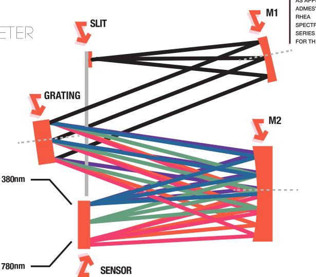
THE ILLUSTRATION BELOW SHOWS THE BASIC PRINCIPLE AND COMPONENTS OF A SPECTROPHOTOMETER'S OPTICAL BENCH AS APPLIED IN ADMESY'S RHEA SPECTRORADIOMETER SERIES FOR THE VIS RANGE.
