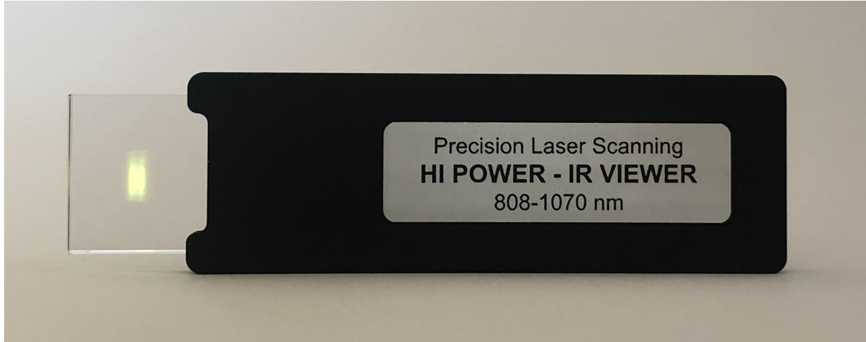
Unretouched image of NIR laser diode with “rectangular” beam
