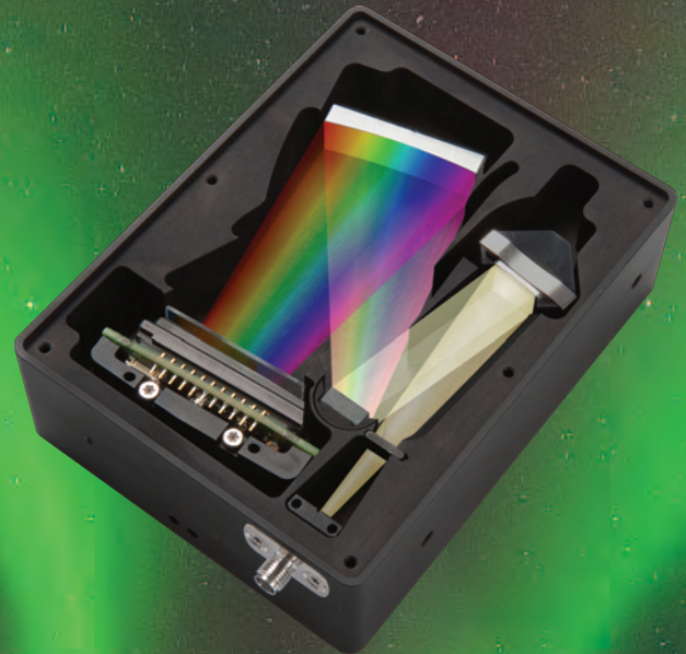
Continuously Variable Order Sorting Filter mounted in front of sensor array for suppression of higher orders and background noise in compact spectrometers (By courtesy of Avantes).
